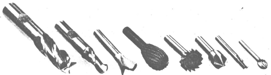
MANY TYPES OF CUTTERS can be used for vertical-spindle machining. Some are shown above. Use milling cutters with care to keep them sharp.
