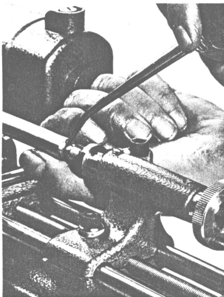
LUBRICATE THE DEAD CENTER with light machine oil and adjust it carefully.
