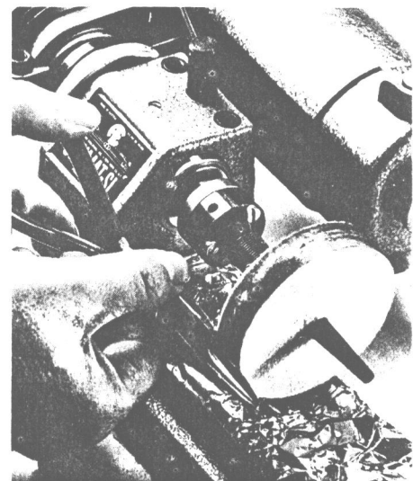
FELT OR RUBBER wheels or polishing points can be screwed on the arbor's tapered shank.
