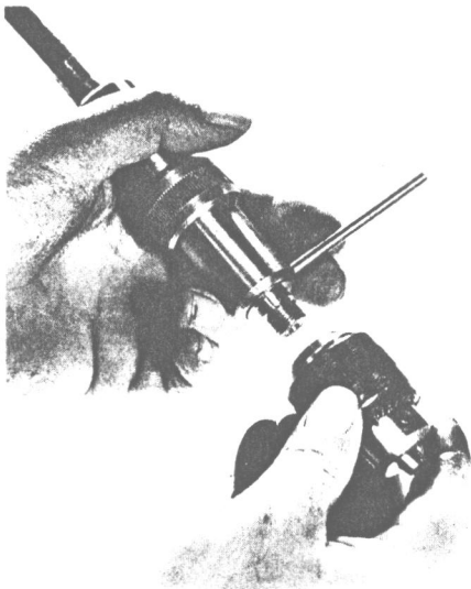
THE SHAFT'S HANDPIECE has the same nose thread as the Unimat's spindle.
