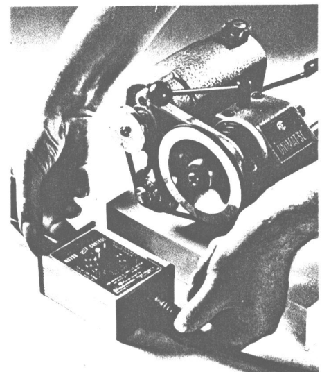
THE ELECTRONIC SPEED CONTROL maintains motor torque through zero-to-full speed range.
