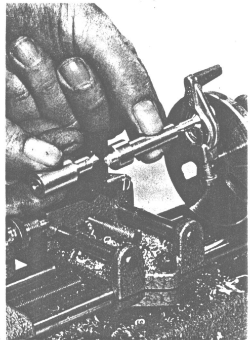
PARTS MAY BREAK before they're finished if you turn end stubs too small in diameter.
